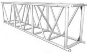
The 30" x 20.5" fork end truss on the Stage Pavilion spans 40'. It is made up of five 8' pieces. The trusses are joined together with 3/4" steel clevis pins through 2" OD steel fork end connections.
