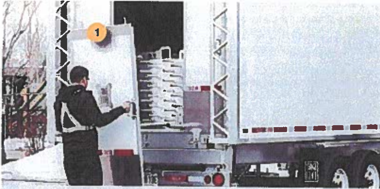
1 New easy access door and integrated storage system under floor panels.
