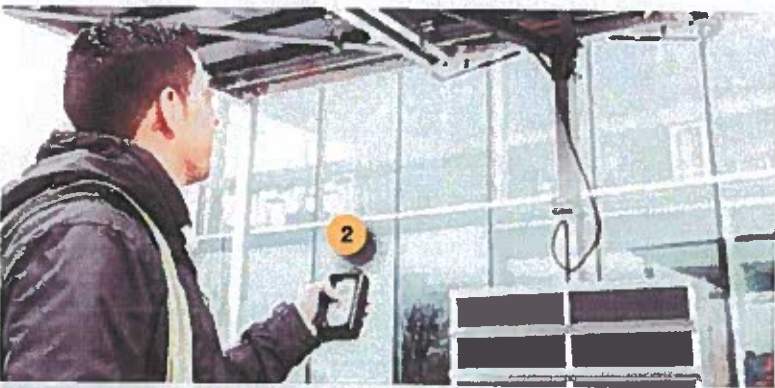
2 Roof raised with a simple operation of the 12v remote controlling the hydraulic lifting mast.
