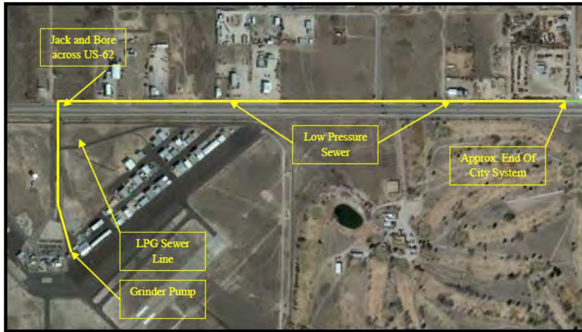
Figure 8 Connection to City of Hobbs SAS System
