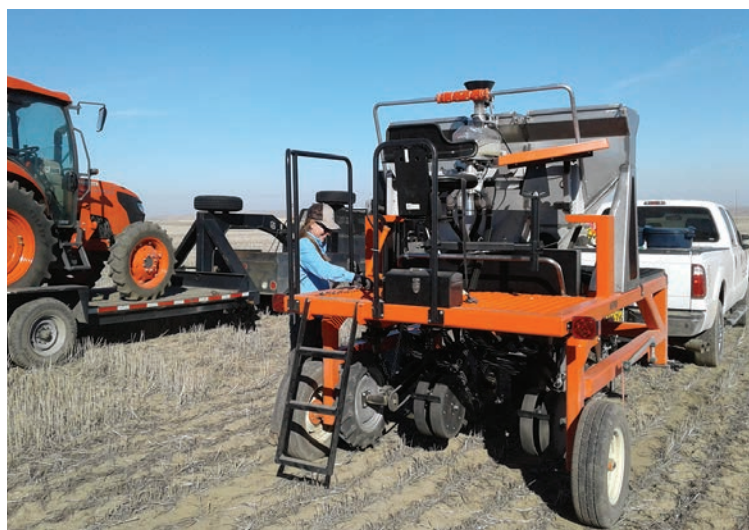
Getting ready to plant at the 2019-2020 Morrow County site. The customized plot drill uses low-disturbance openers. Dry fertilizer is placed into a band below and in-between paired rows. Seed (or fertilizer) can be “run through” stainless steel hoppers or an extremely accurate metering device controlled by the operator. Photograph by Larry Lutchter.
