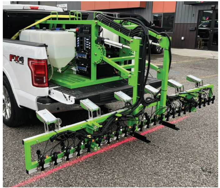
Custom built Weed-It system. The red light causes plants to photosynthesize and individual nozzles are activated. The sensor is being assessed for discriminating chlorophyll content among weeds and wheat.
