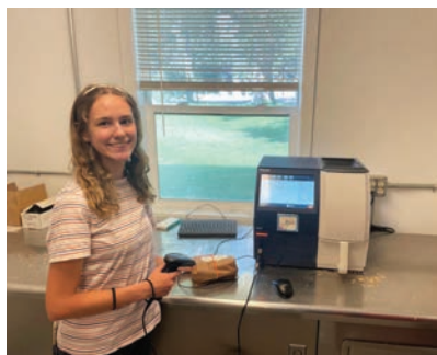
Student worker Sydnee Enright scanning barcoded grain samples for the near infrared spectroscopy analysis for moisture, protein, and test weight.
