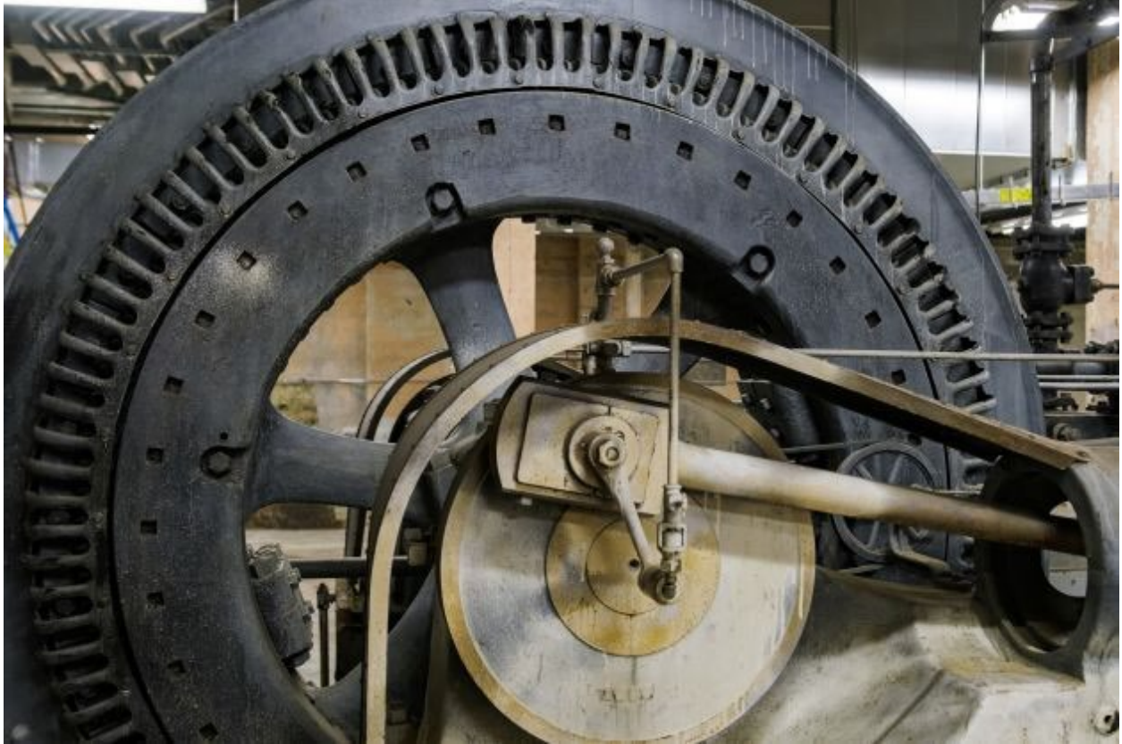
The heart of the system "Old Joe" which is a giant electrical motor with two pistons still exists in the sub-basement.
