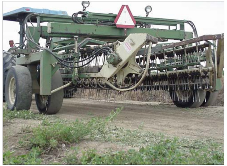
Alfalfa Rake tines 7" off the ground
