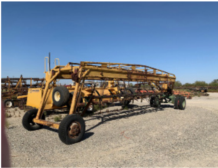
Carryall 40.5 ft long x 10.5 wide Implement being transported often 4 - 5 ft wider
