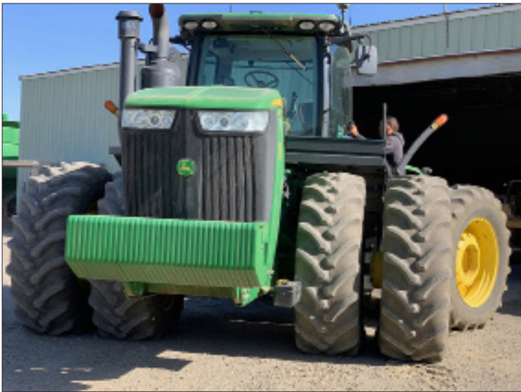
John Deere 9410R Tractor with Duals 15'2" wide, 17' 6" with step
