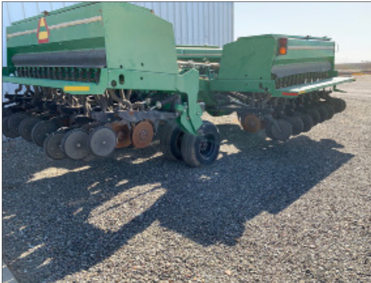
Grain drill folded into three sections Side 1 Folded 26 ft long by 21 ft wide
