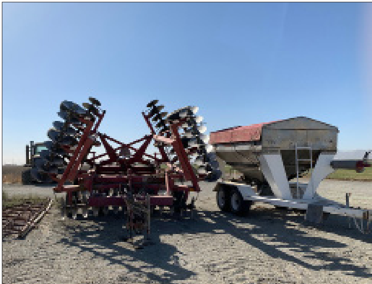
Stubble disc folded 3 ways 25.5 ft wide, 11 ft long folded
