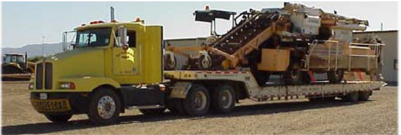
Lowbed hauling tomato harvester Trailer length 418/2" Trailer clearance 16" Front truck axle to rear trailer axle 52'4"
