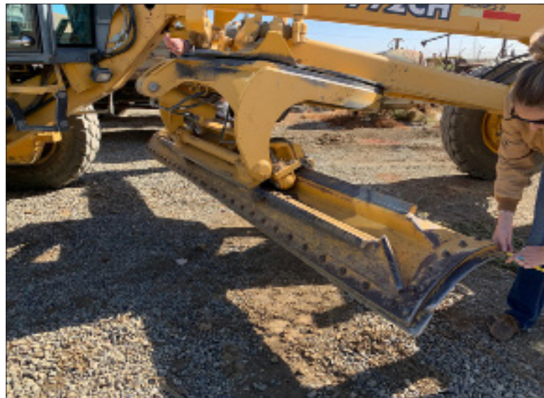
Road Grader and Blade Grader 30'3" long Blade 14'1" wide
