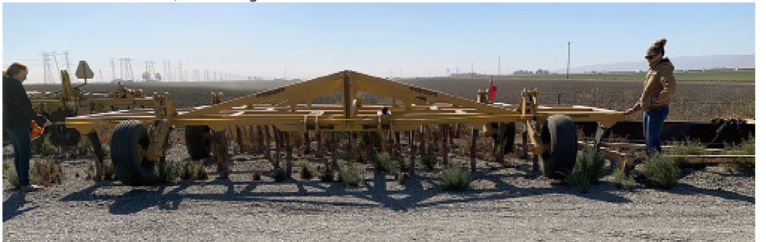
Chisel plow - can't be folded - blades very close to ground 11 ft long by 25 ft wide
