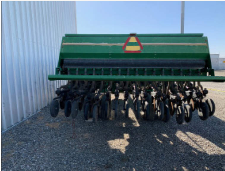
Grain drill folded into three sections Middle Section Folded 15 ft wide
