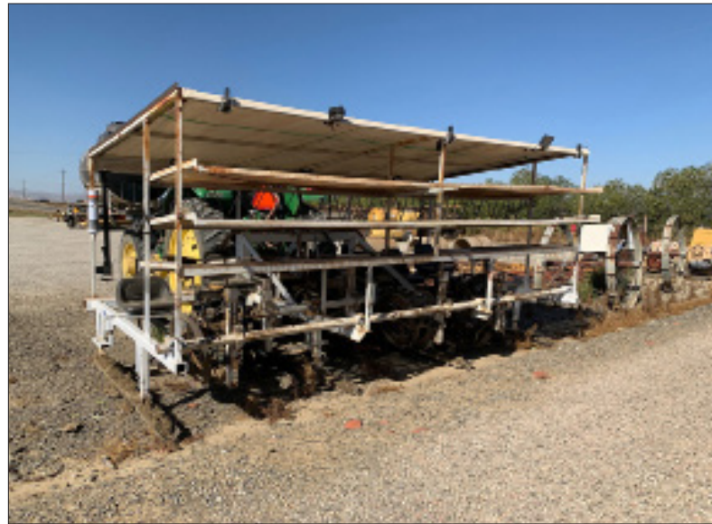
Planter Sled 15 ft wide 6 - 8 inches off the ground
