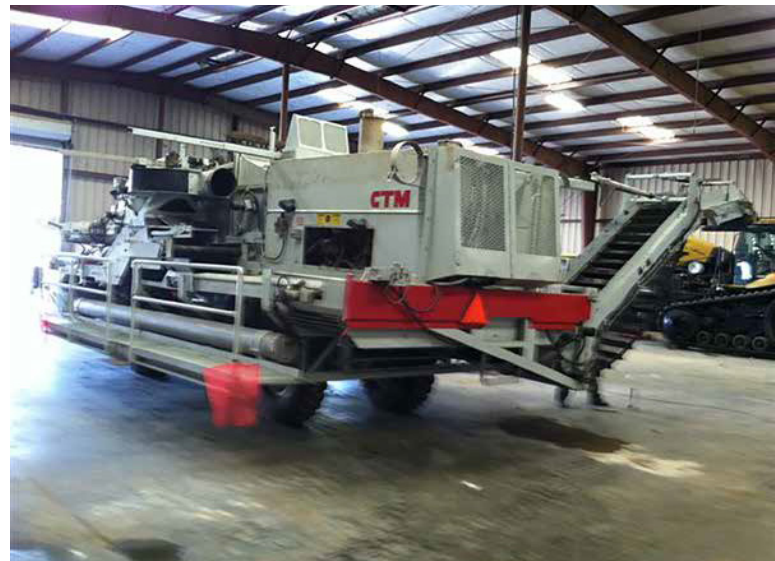
Tomato Harvester – wheels set for 60" beds. 54' long x 11 ft wide, plus elevator
