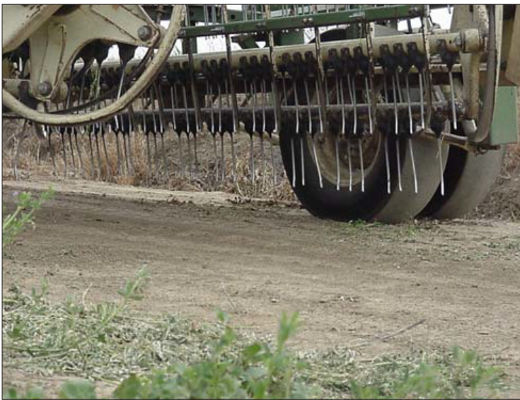
Alfalfa Rake 12 ft long, 5.5' from rake to tractor hitch
