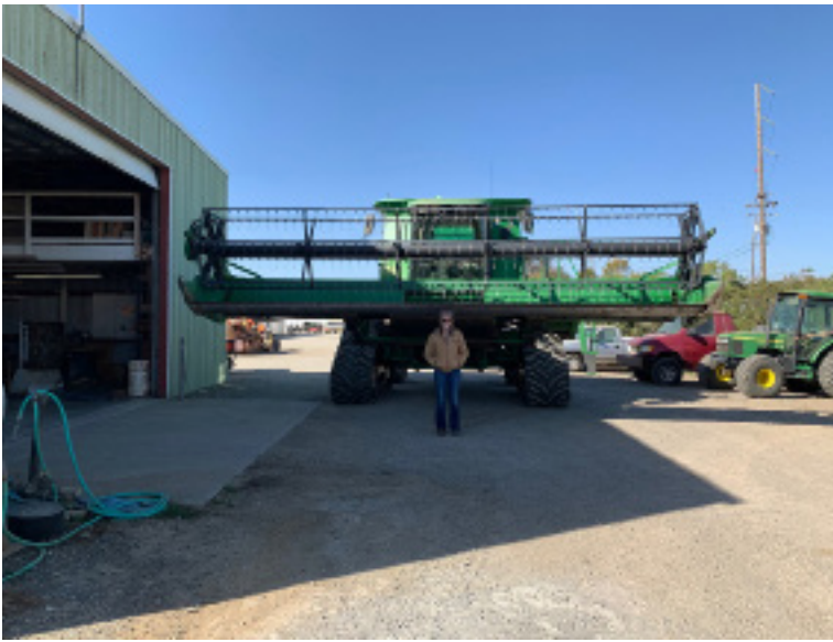
John Deere Harvester with header attached 26.5 ' wide by 17'6' tall 31t front to back
