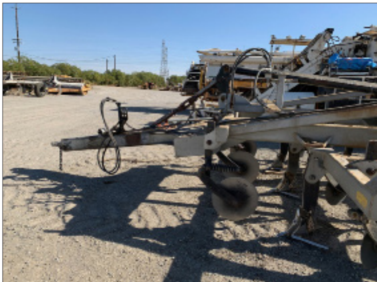
Implement to rip alfalfa and chisel-Front Section See back section above 2 of 3 photos
